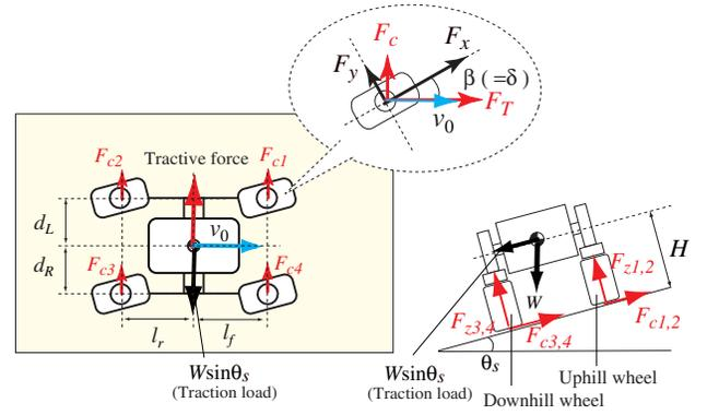
Fig. 3. Force balance on slope traversing case
