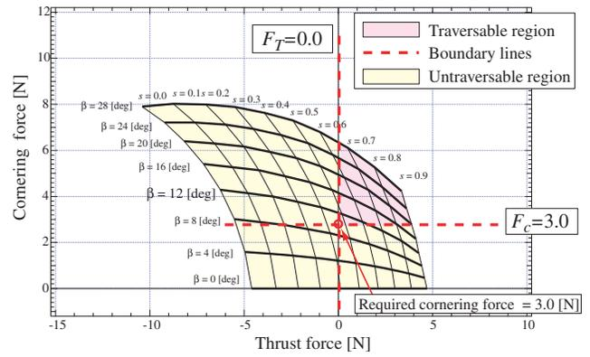
Fig. 8. Thrust-Cornering Characteristic Diagram
