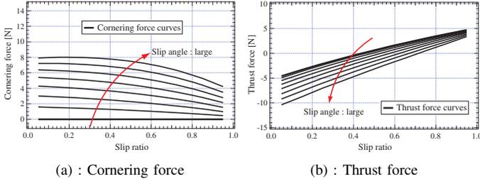
Fig. 7. Characteristics of cornering and thrust forces
