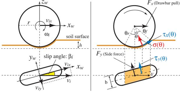
Fig. 4. Analytical model for wheel force
