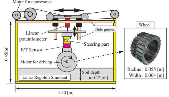
Fig. 5. Schematic view of single wheel test bed
