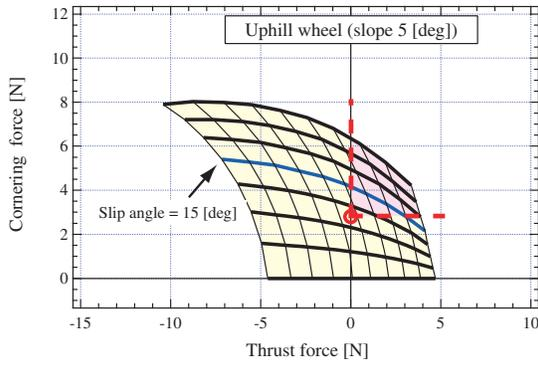
Fig. 11. Thrust-cornering characteristic diagram : case-A (slope angle is 5 [deg])
