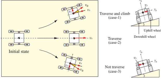
Fig. 2. Slope traversing case: traversable and untraversable
