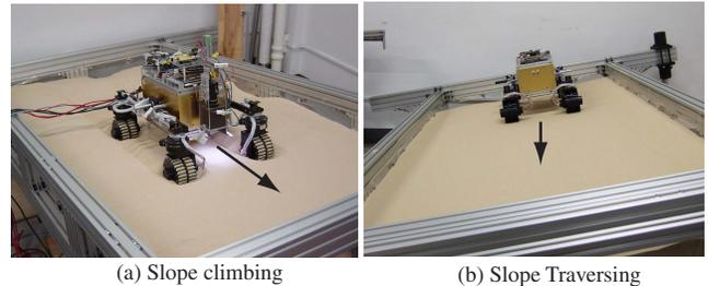
Fig. 1. Definition of slope climbing/traversing cases
