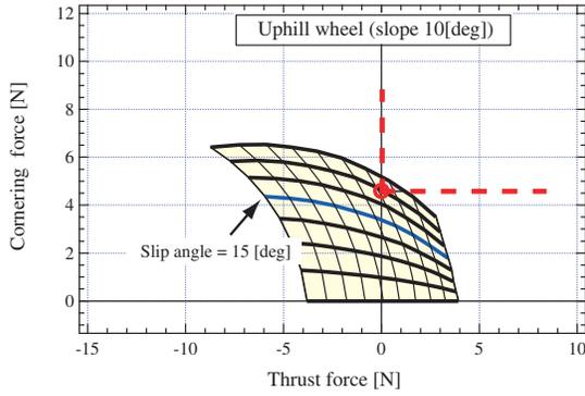
Fig. 12. Thrust-cornering characteristic diagram : case-B (slope angle is 10 [deg])
