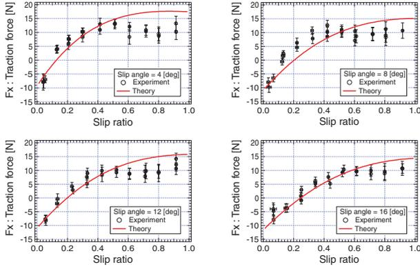
Fig. 8. Experimental results (slip ratio - traction force)
