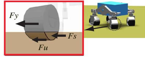
Fig. 4. Lateral (side) forces acting on the wheel
