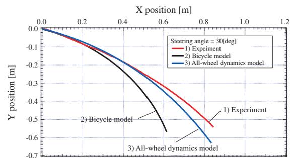
Fig. 12. Trajectory comparison of the experiment and the simulation
