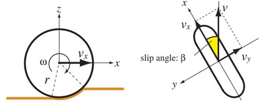
Fig. 2. Wheel coordinate system
