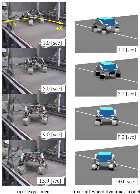
Fig. 11. Comparison of the rover's steering motion
