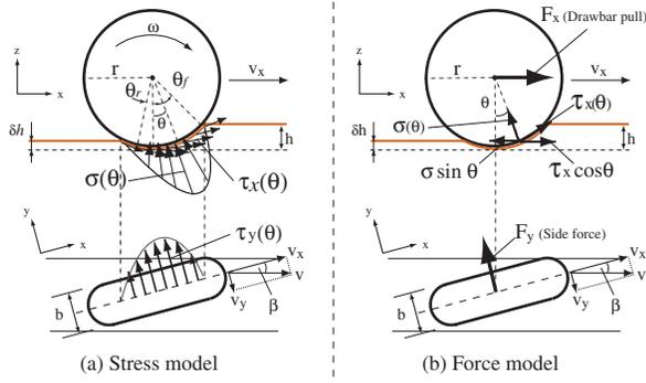
Fig. 3. Wheel contact model on loose soil
