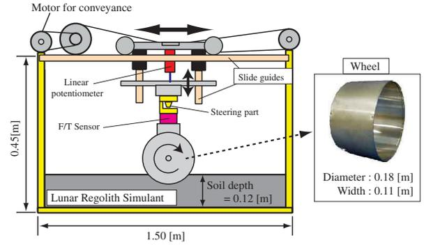
Fig. 7. Schematic view of the single wheel test bed
