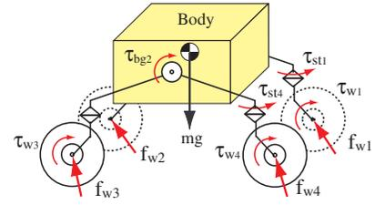
Fig. 10. Dynamics model of the rover
