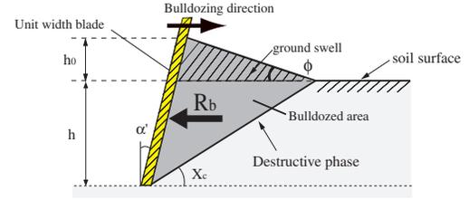
Fig. 5. Estimation model of bulldozing resistance
